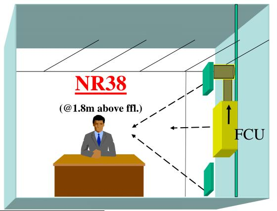
FCU @ 210 l/s & 30 Pa With room absorption, ductwork, plenum & grille. Note, lower air volume due to lower on coil temp. Generally lower cooling performance if vertical FCU are compared with horizontal ceiling mounted FCU.
