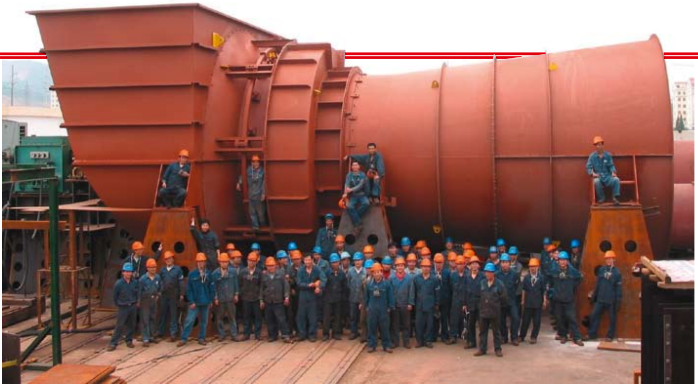
Assembly of a 6 megawatt mixed-flow fan.
